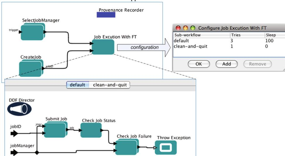
Fig. 6. Fault tolerance and provenance support in Kepler workflow.
