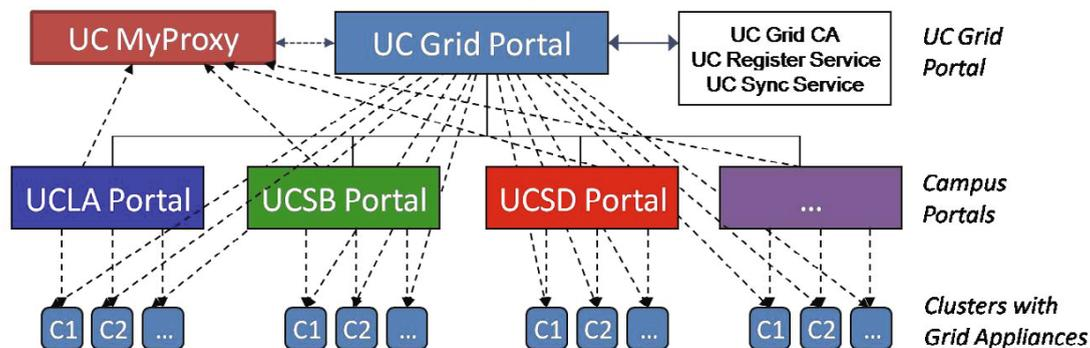
Fig. 1. The architecture of the University of California (UC) Grid.
