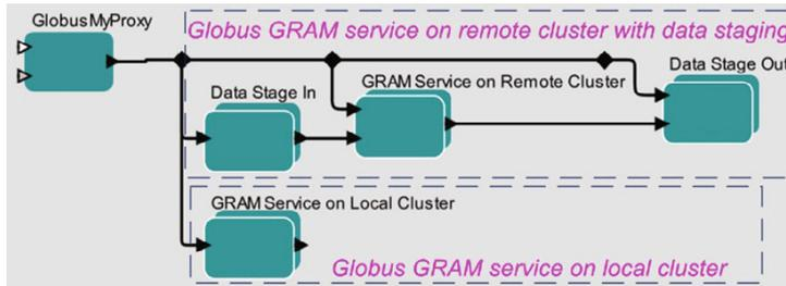
Fig. 5. Kepler workflow for enzyme design processes on multiple clusters. The GRAM service composite actor will invoke the workflow shown in Fig. 4 on the target cluster.
