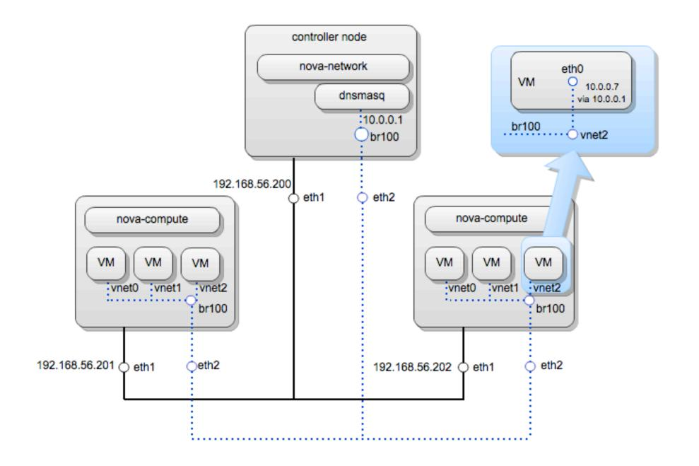
**eth1** is the management network interface (controlled by --public\_interface). The controller has address 192.168.56.200, and we have a default gateway on 192.168.56.101
