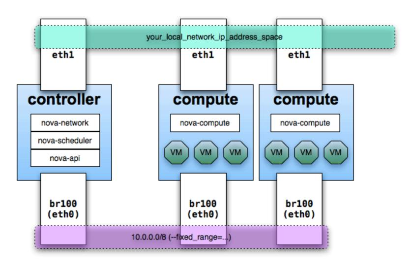
Flat DHCP network, multiple interfaces, multiple servers with libvirt driver
